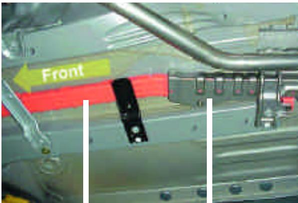
Orange Plastic Shield      Thermal Shield
